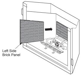
Figure 44 - Installing Side Brick Panels
